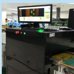
4. AOI inspection after soldering
