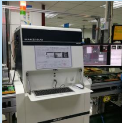
2. AOI inspection before soldering
