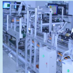
5. Automatic screwing & labeling
